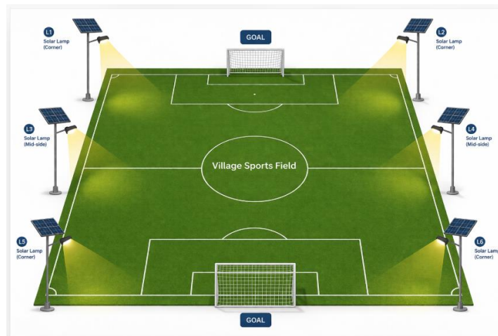
Figure 3. Solar Lamp Placement Design in the Field.
