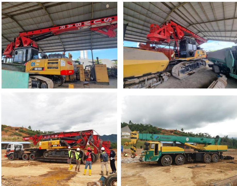
Gambar 3. Alat hydraulic drilling rig, service crane (Proyek di Sumatera Barat).
